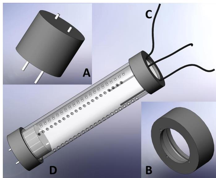
**Appendix 2.** Individual parts of the SOFT system. A) Rubber stopper with 2 integrated steel channels B) Upper cap with 3 small holes to guide tubing for aeration and seawater inflow/outflow C) Iso-versinic tubing D) Assembly of individual parts with the core liner.
